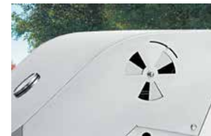
AIR/TEMPERATURE CONTROL LOUVERS
