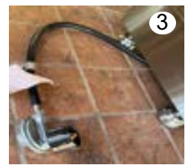
3 Pass the regulator hose between the legs of the Appliance.
