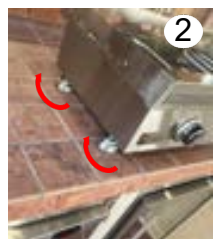
2 Adjust the level of the unit by unscrewing the adjustable feet.
