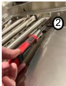
2 Remove the screw under the burner
