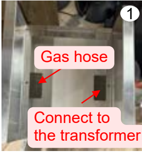
1 Remove the feet and connect the gas line. (See page 16 - 19).
