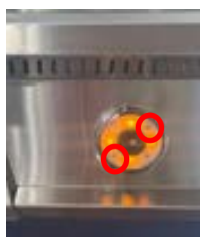
Remove the SLOTTED screws circled in red. DO NOT UNSCREW THE TWO PHILLIPS
