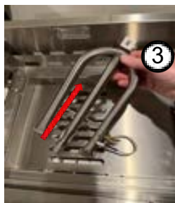
3 Remove the burner
