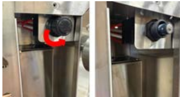
Unscrew the cap and remove the battery then install the new one in the same way and screw the cap.
